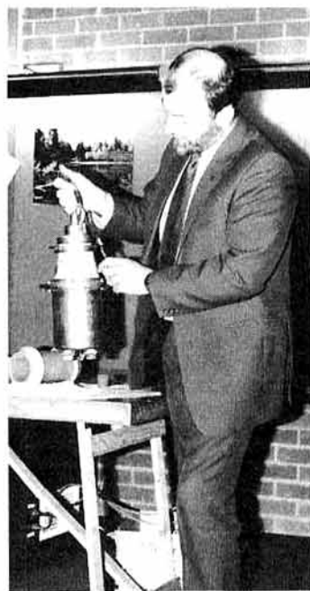
Andy, G0JXM, gave an illustrated talk and demonstration on the industrial uses of RF and induction heating to members of the Cheltenham ARS, recently. The photograph (above) shows Andy holding a water-cooled RF power triode which has an output of 166kW at frequencies up to 30MHz. Some members of the club were entertaining thoughts of using the valve in a linear amplifier until Andy pointed out that it need 4kW to drive it and costs in the region of £3,000. Oh well, back to the drawing board....
