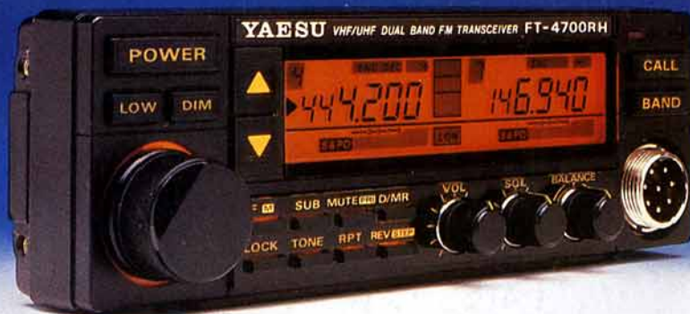
FT-4700RH control head (1 15 / 16 " x 5 7 / 8 " x 1")
